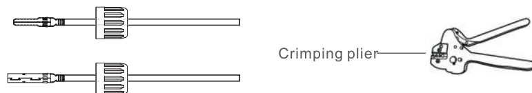
▲ Figure 5.14 Crimp the contact pin to the wire
