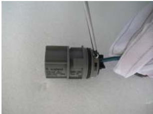
▲ Figure 4.16 Connect Wires to the Terminal
