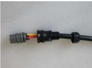
▲ Figure 4.16 Connect Wires to the Terminal
